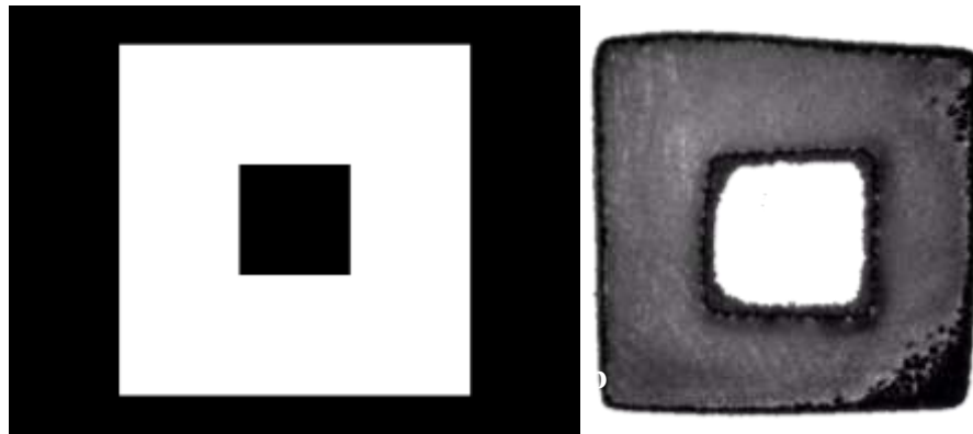
Figure 5.1 - A sintered interior square. On the left a) the reference image and b) the resulting sintered part. Due to non-uniformity in the projector power distribution the part showed high degrees of asymmetry, with the lower right corner not fully fusing to the layer below while the upper left corner melt pool overran its boundaries significantly.
